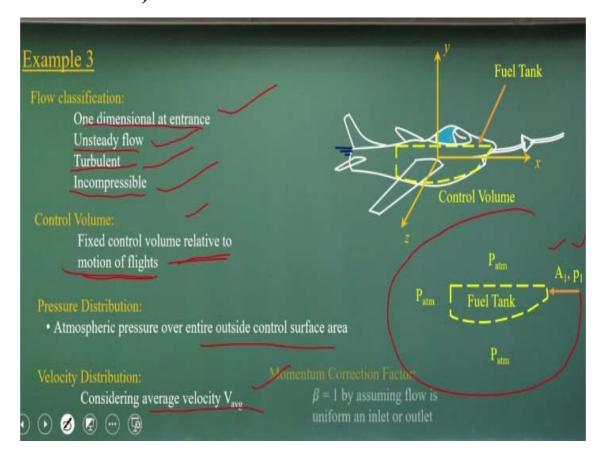
And if I define the fuel tank and this coordinate of x, y, z the problems can be considered is one dimensional. Fluid is unsteady flow, but we can simplify it make it the steady flow; turbulent, incompressible. So these three conditions will be there; one dimensional, we are not considering the velocity distributions and all. The unsteady, turbulent and incompressible flow. That is what the classifications.
