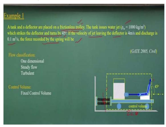
Now, let us come it to solve example one which is GATE 2005 civil engineering problems. The problem is that there is a tank or deflectors are placed in a frictionless trolley. Okay, there is no frictions components, okay. The water issues the water jet which is have a the density of the water is 1000 kg per meter cube. It strike to a deflectors, turn 45 degree.
