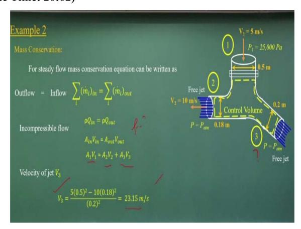
Then we will apply mass conservation equations that let us apply mass conservation equations to compute it what could be the velocity at the section 3. So we are applying the mass conservation equations for these control volumes that to compute what could be the velocity at this point. So if I apply this mass conservation equation which are very simple form is rate of mass influx into the control volume is equal to rate of the mass outflux from this control volume.
