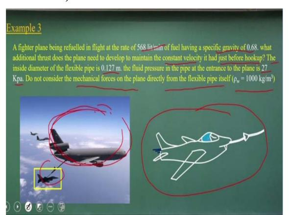
Let us take another example. A fighter plane being refueled in a flight at the rate of 568 liter per minute of fuel having specific gravity of 0.68. What additional thrust does the plane need to develop or maintain constant velocity it had just before hookup. The inside diameter of the flexible pipe is 0.127 meters. The fluid pressure in the pipe at the entrance to the plane is 27 kilo Pascal.
