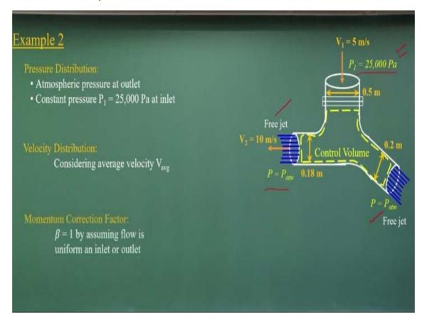
So if we have this fixed control volumes, first we will find out that the pressures. The pressures at the inlet is given is 25,000 Pascal. At the outlet is pressure is atmospheric pressure. That what is there. So you have the free jet at these two locations where pressure is the atmospheric pressures. At these two point you have a pressure equal to atmospheric pressure, but at this point I have the pressure which is 25,000 Pascal, Newton per millimeter square.
