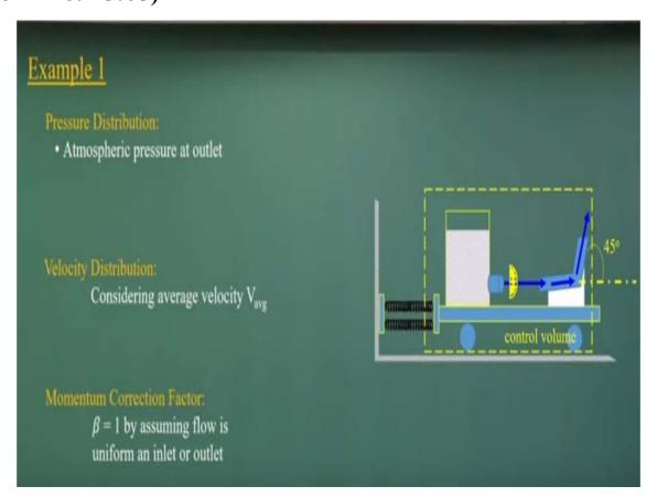
So the pressure distributions at the outlet will be the atmospheric pressure. Here also we have consider the velocity distributions again average velocity. No doubt there will
