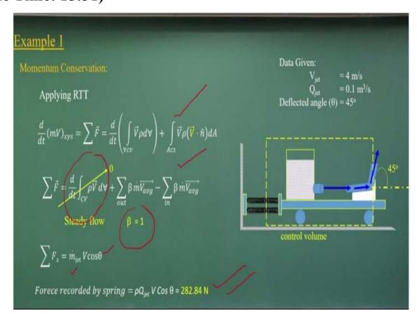
Now let us apply the directly the momentum conservation equations here. If I apply this momentum conservation equation this some of the forces should equal to the rate of the change of momentum flux within the control volume is equal to the net outflux of momentum flux passing through these control surface.
